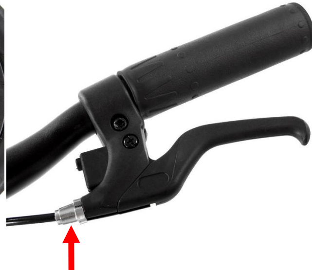
fine-tune the brake nut
