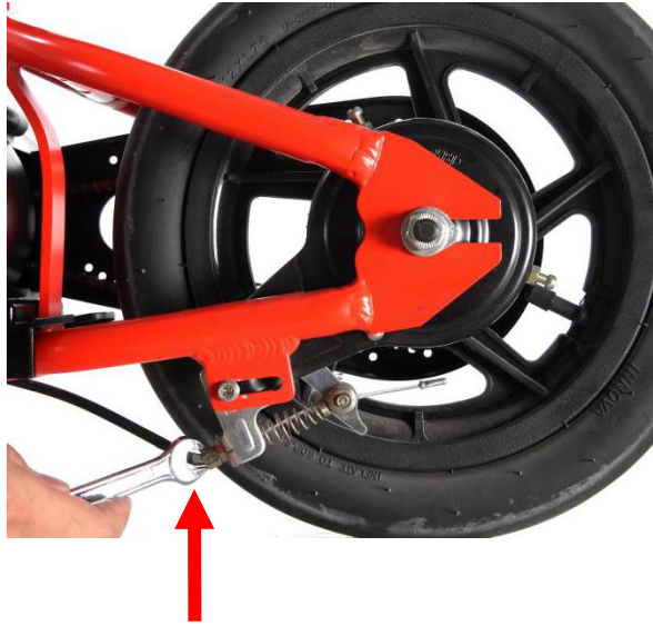
fine-tune the brake nut
